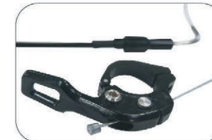
4. Insert the cable into the cable housing.
